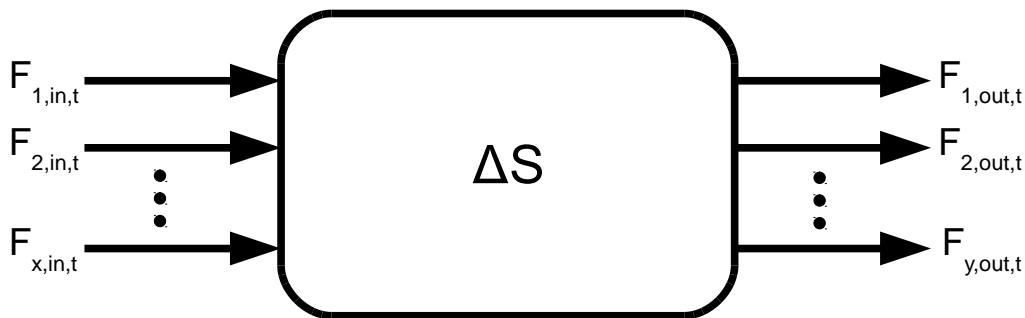
Figure 1: Simple balancing layout. Several fluxes may enter or leave a system, accumulation ( \Delta S ) is possible.
