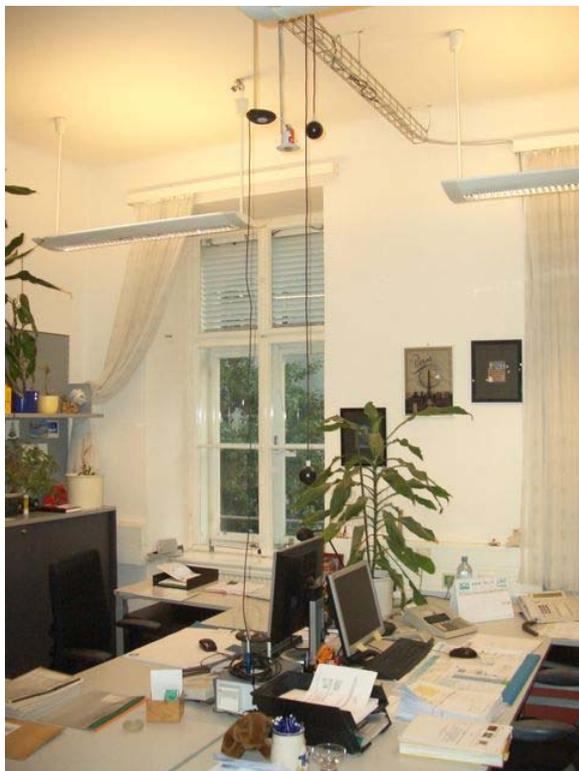
Figure 4 Workplaces in R2 with motorized window, internal venetian blinds and sensors
