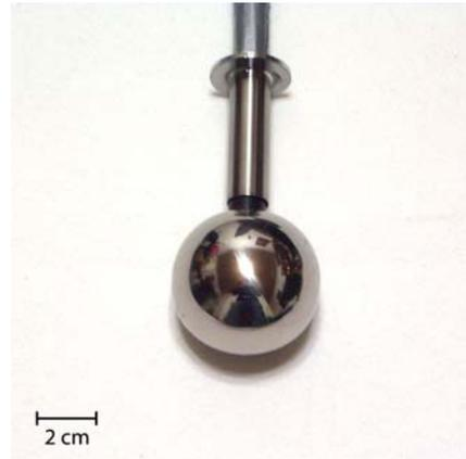
**Figure 2:** Example of the sphere shaped sensor used to determine mean radiant temperatures
