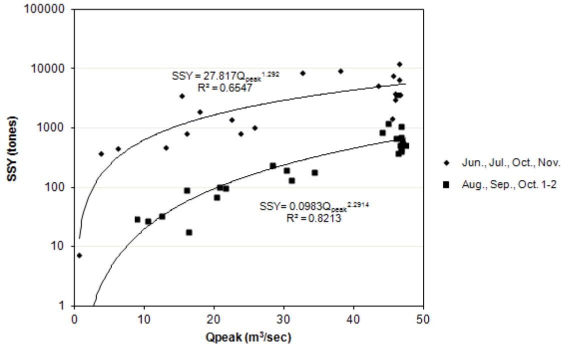
**Figure 3-8: Sediment rating curves based on  $Q_{peak}$**
