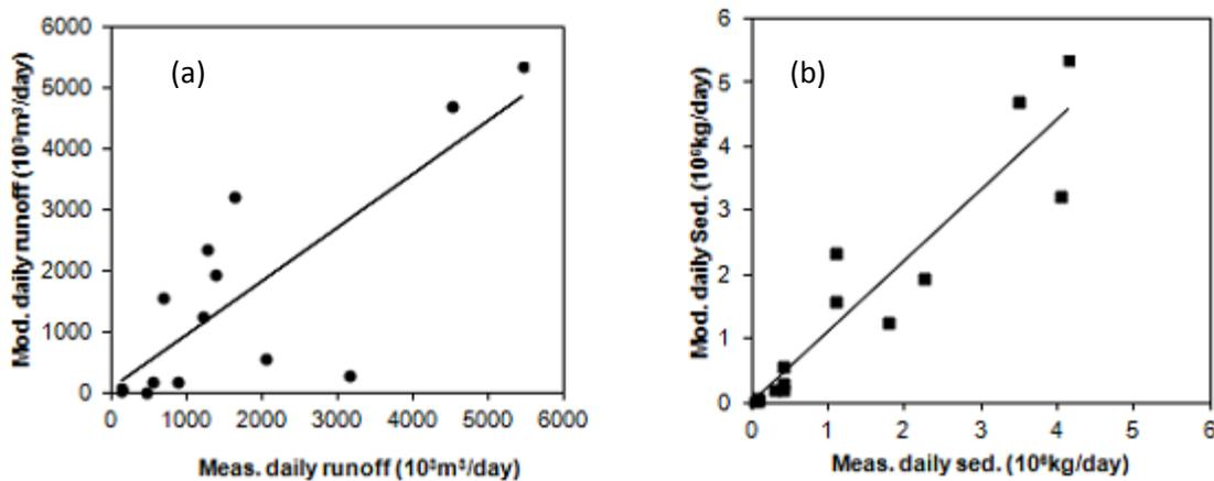
**Figure 4-3: Model validation results on daily runoff (a) and sediment (b) for the year 2013 for selected days in the time period 19/6/2013 to 29/9/2013**
