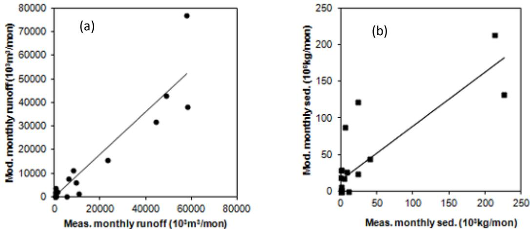
**Figure 4-4: Model validation results on monthly and measured runoff (a) and sediment (b) data throughout the two years simulation period**
