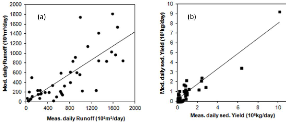
**Figure 4-2: Model calibration results on daily runoff (a) and sediment yield (b) for selected days in the time period 5/10/2011 to 8/10/2012**
