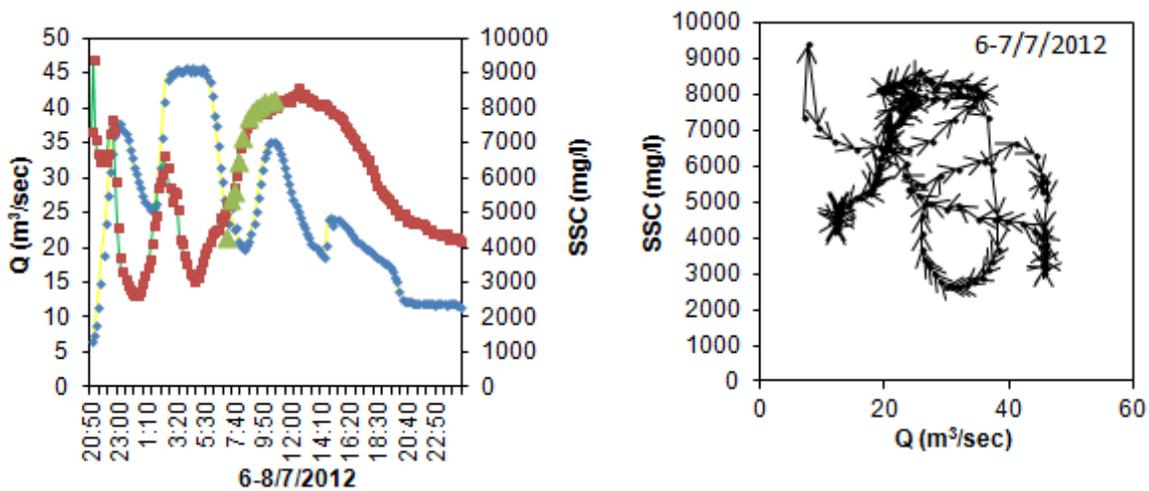
Figure 3-5: SSC-discharge hysteresis loop of a complicated pattern
