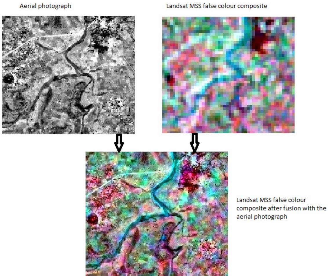
**Figure 2-4: 1979 Landsat MSS false color composite of small part of the area around the .outlet of the Koga catchment before and after pansharpening**
