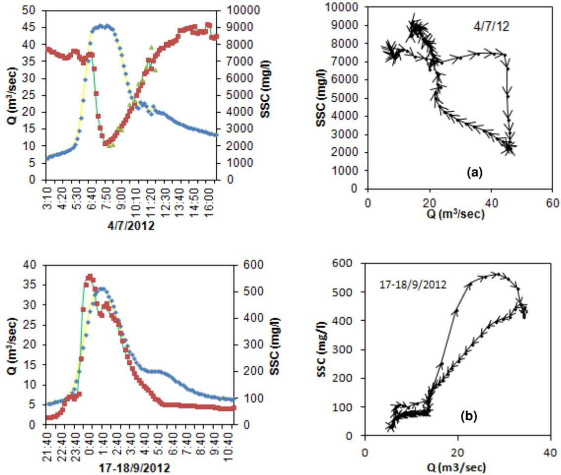
Figure 3-4: SSC-discharge hysteresis loops of (a) CAC and (b) clockwise patterns
