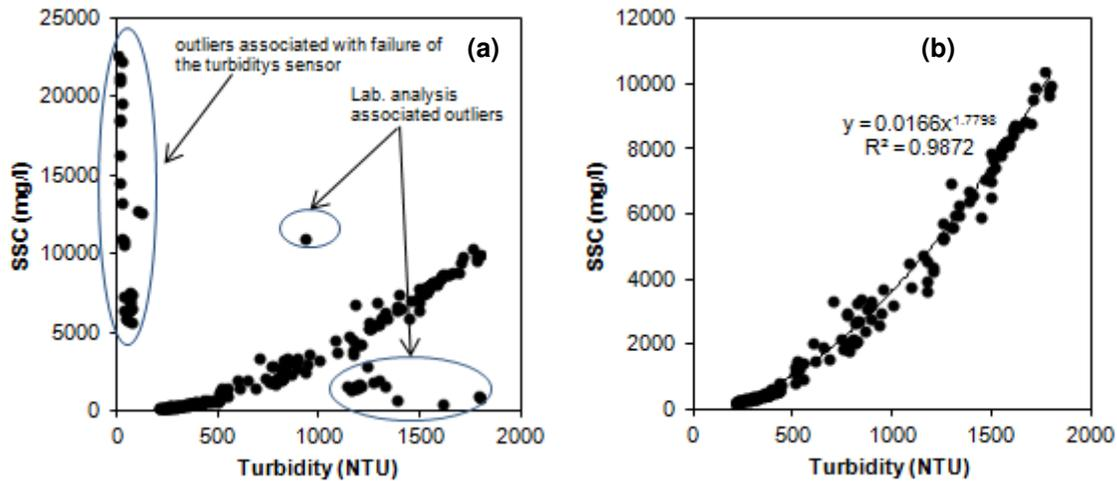
**Figure 3-2: SSC-Turbidity relationship before (a) and after (b) removing outliers**
