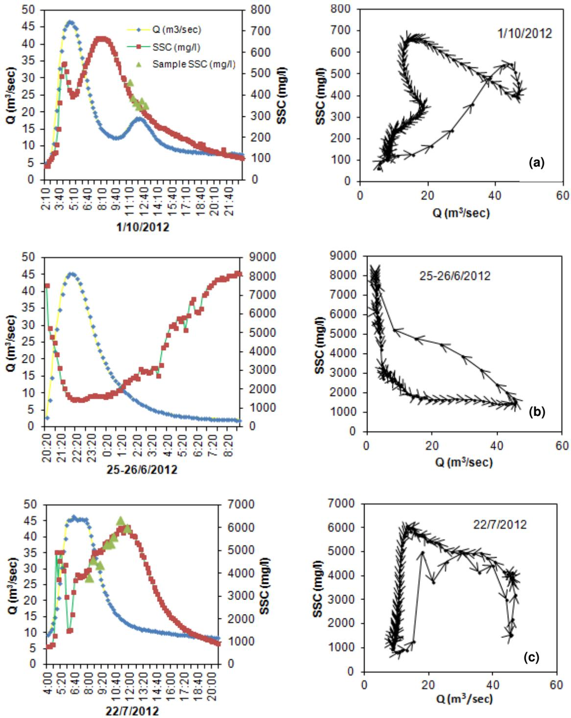
Figure 3-3: SSC-discharge hysteresis loops of (a) ACA; and (b & c) anticlockwise patterns of some of the events
