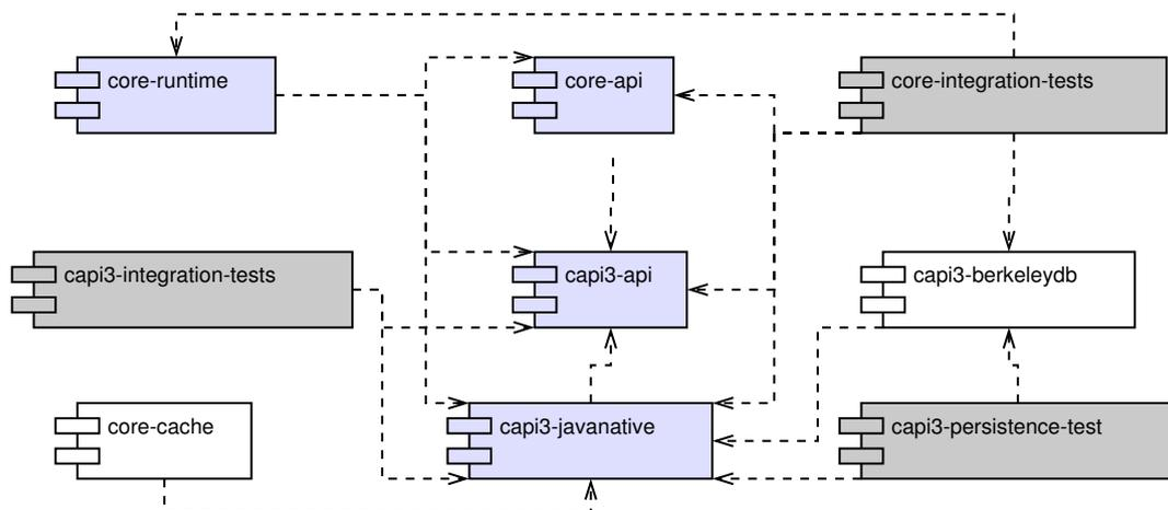
**Figure 5.1:** Components of MozartSpaces relevant to the persistence and dependencies between them. Blue components are always deployed and used at runtime, gray components contain only test cases and are never used at runtime and white components can be optionally used at runtime if their functionality is required.
