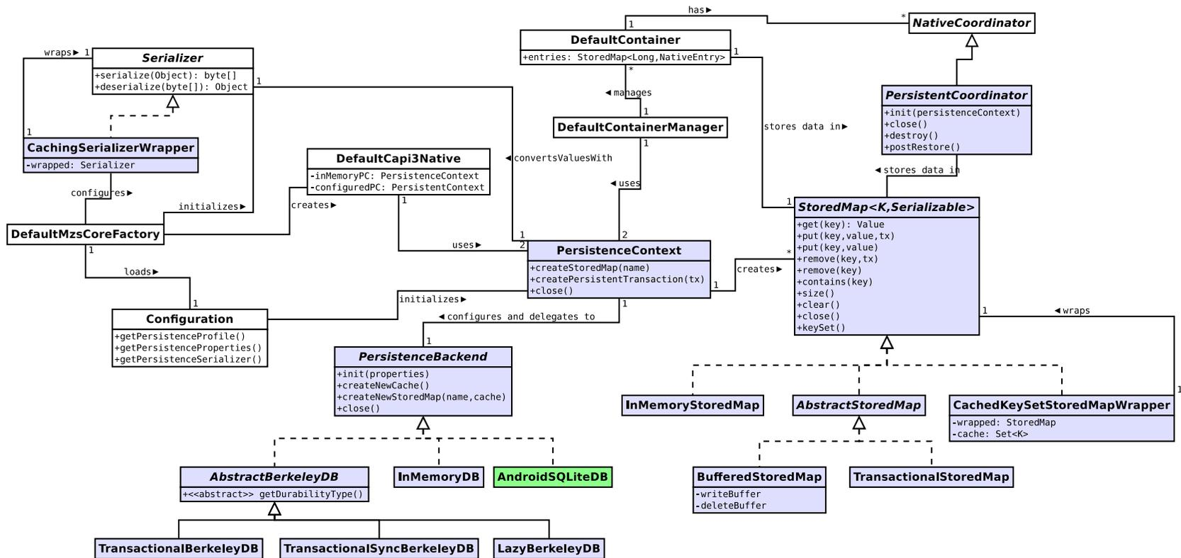
**Figure 5.2:** Class diagram with the most important classes and interfaces of the persistence layer. Classes that already existed in previous versions of MozartSpaces are white, new classes are blue and classes specific to the Android version are green.
