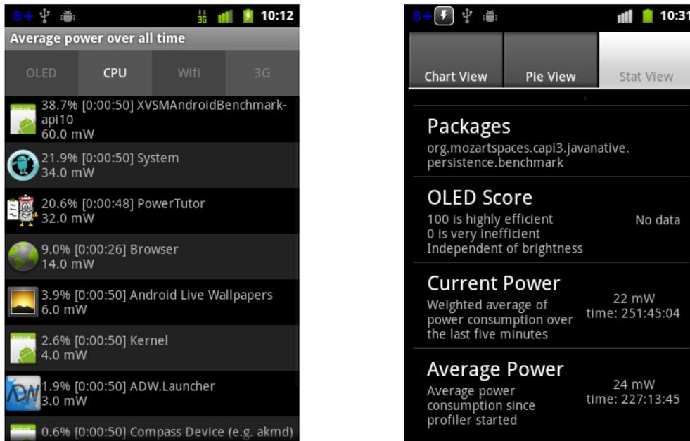
**Figure 5.8:** PowerTutor showing current energy usage per application (left) and per hardware component (right)
