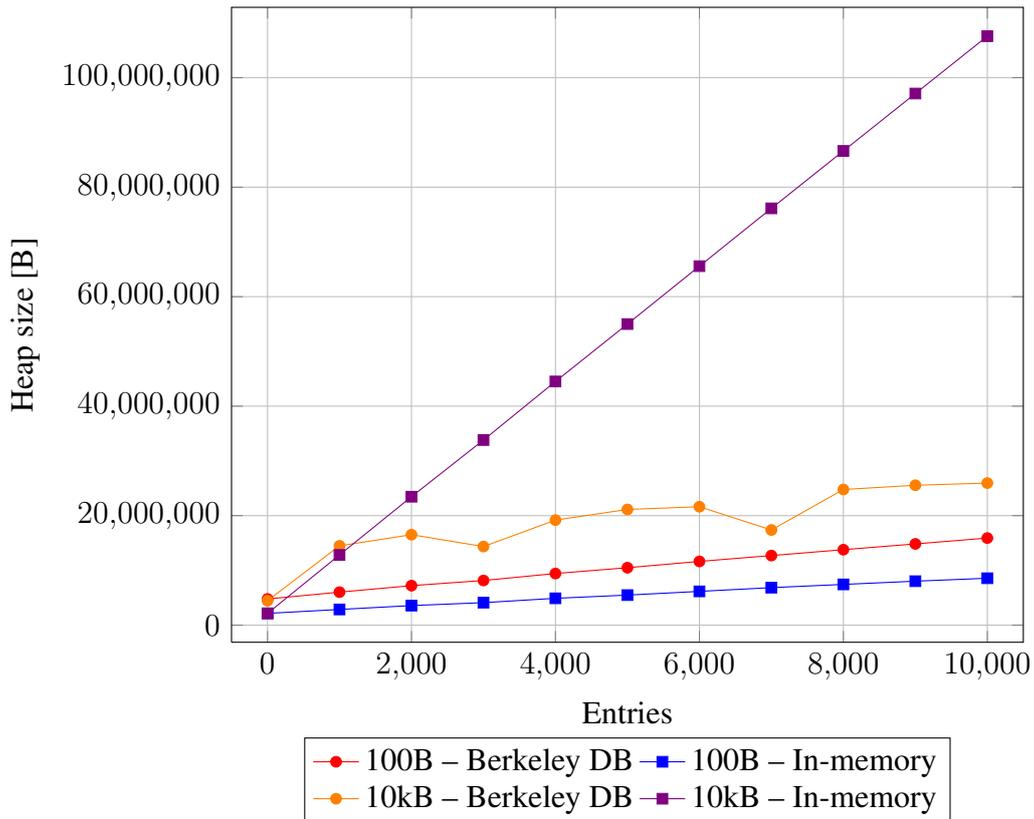
**Figure 6.4:** Memory usage of MozartSpaces with the In-memory profile and with the Transactional Berkeley DB profile
