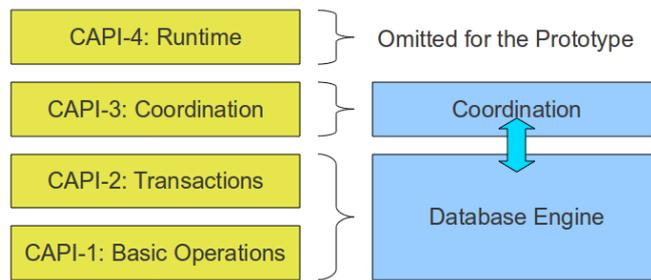
**Figure 3.1:** Architecture of XVSM implementation based on a database [Bar10]
