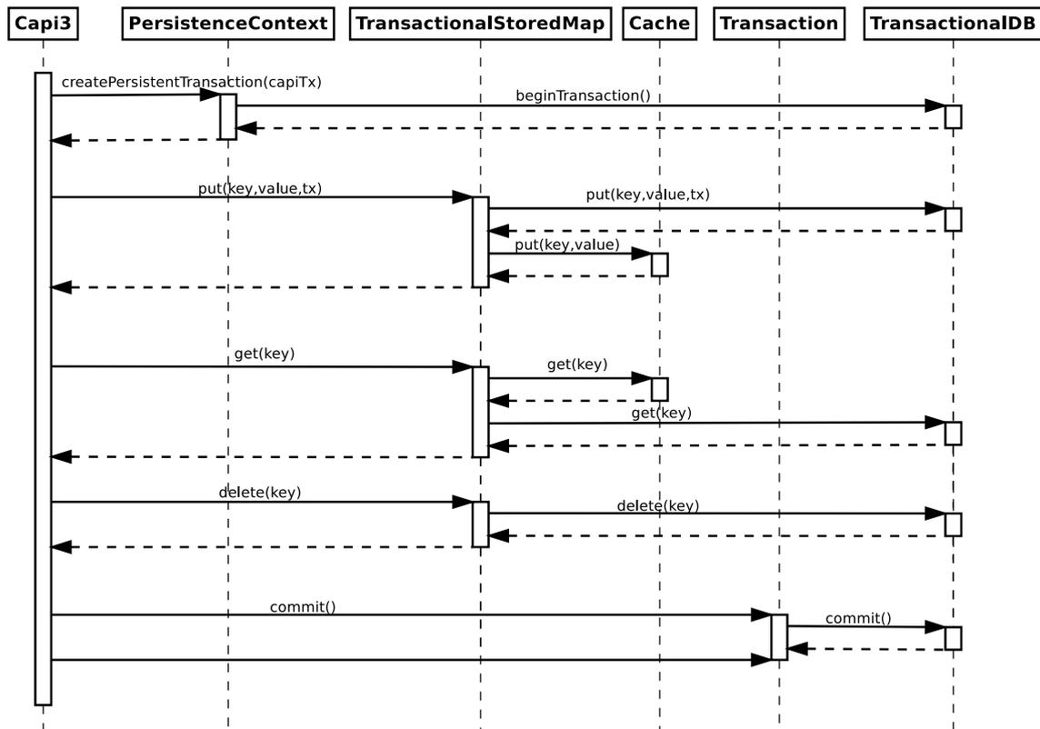
**Figure 5.6:** Sequence diagram of TransactionalStoredMap
