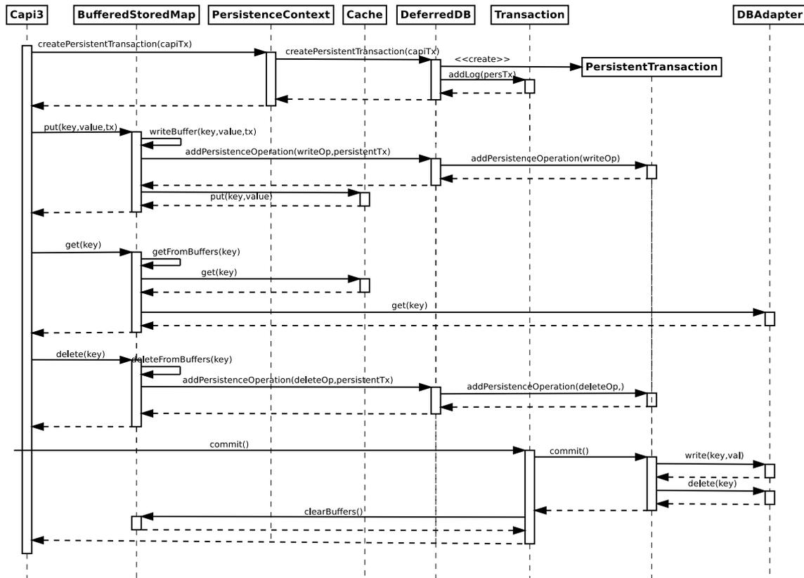
Figure 5.5: Sequence diagram of BufferedStoredMap
